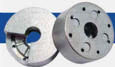
Figure 5: A complex undercut feature made possible with the application of In-coring
